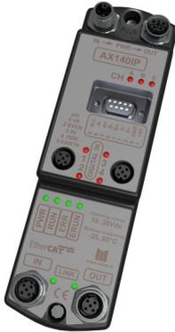
AX140IP is an EtherCAT slave module with an isolated input to read incremental encoder; the encoder is supplied directly from the module. Four digital inputs are available to read proximity, switches, push-button etc. Diagnostic leds indicate EtherCAT connection status, digital input and encoder status.
